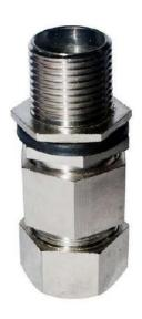
The double compression cable gland is normally designed for all armoured and unarmoured cables to provides compression for both on the cable armoured and inner sheath, it provides strain relief and electrical continuity for the electrical cables throughout.
