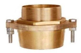
Flange Type Cable Glands are made out of brass castings and are machined accurately to the required sizes. These glands are suitable for armored cables and are called mechanical glands hence suitable for outdoor application.
